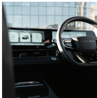
12.3" LCD Driver Cluster & 12.3" Center Control LCD Screen
